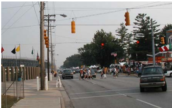
Figure 6-19 At-Grade Pedestrian Crossings Adjacent to a Venue Gate
