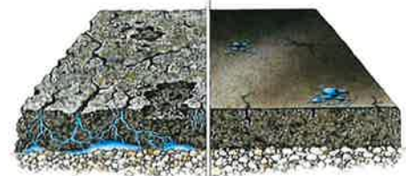
Asphalt Chip Seal Before/After
